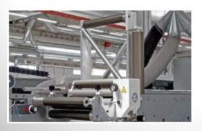
» Unit that separates the release liner from the self adhesive material to allow printing on the adhesive.
